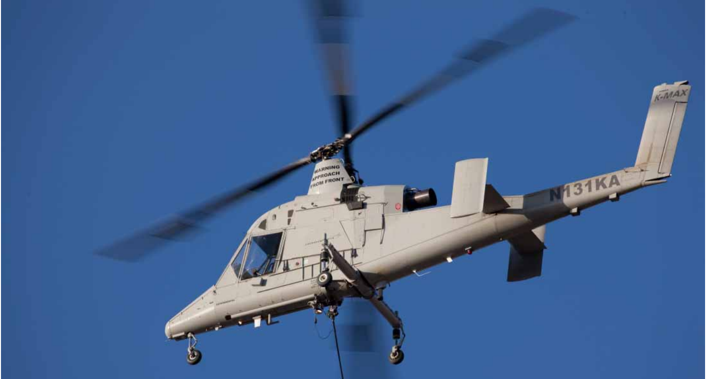
Lockheed/Kaman K-MAX UAT, N131KA, undergoing pilotless flight testing in Yuma, Ariz. (Lockheed photo)
