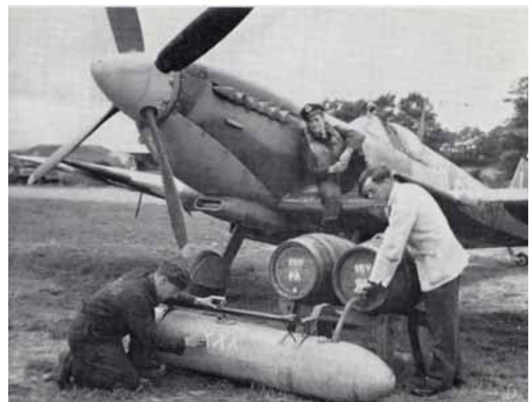
A Mod XXX tank being prepared for shipment. This photo was likely staged in that hanging the tank after filling would have required a lot more effort than if it were filled after it was mounted on the aircraft.
