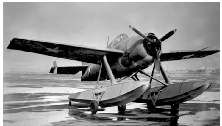
An unusual Grumman Wildcat. BuNo 4038 started life as an F4F-3 but was converted to an F4F-3S floatplane for test and evaluation. Seen here on February 12, 1944. (AAHS photo archives, AAHS-394)
