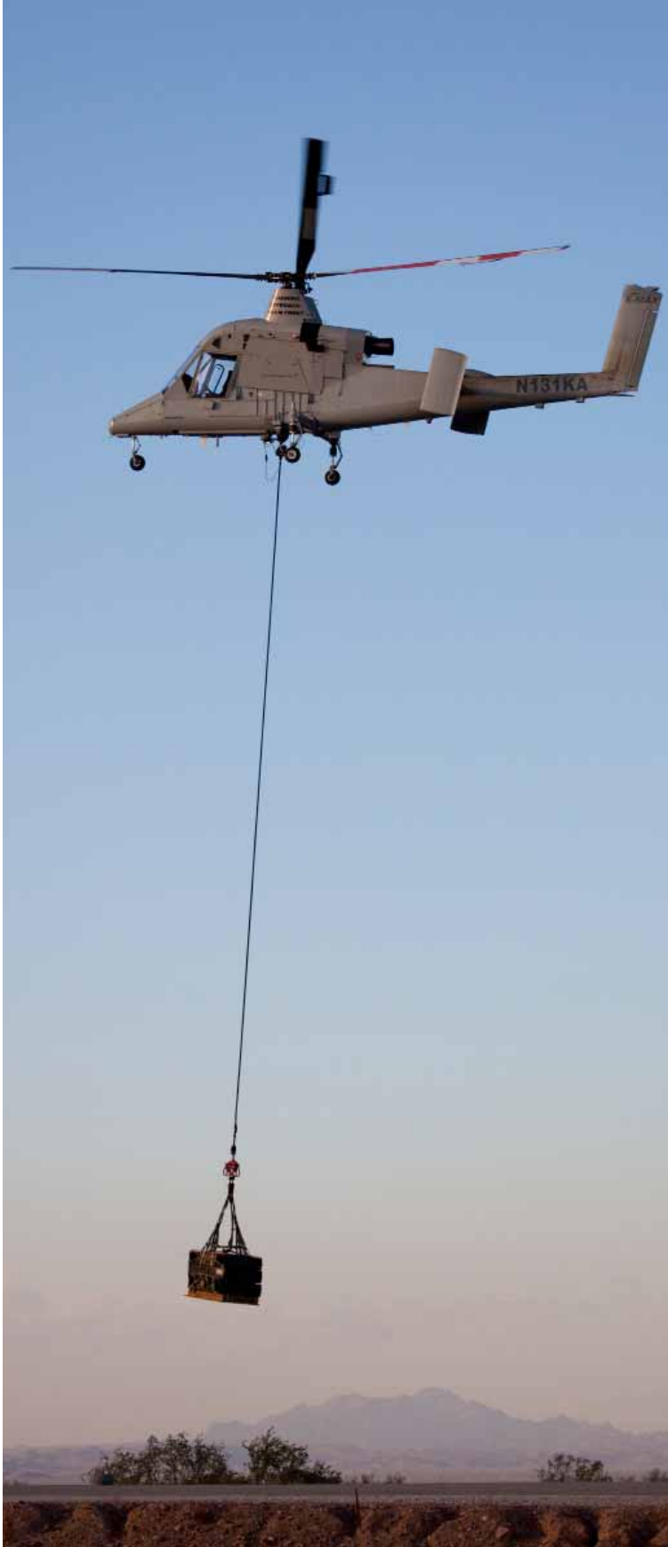
Lockheed/Kaman K-MAX UAT, N131KA, picking up a pallet load during flight testing in Yuma, Ariz. (Lockheed photo)
